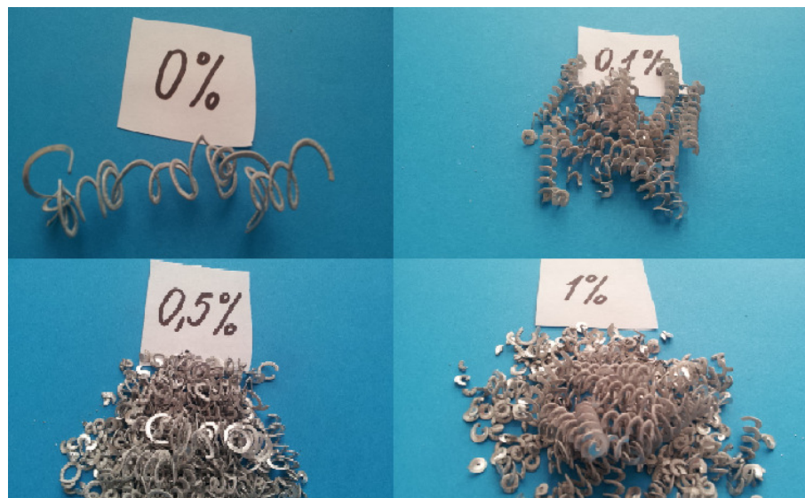
Fig. 3. Shape and chip size in AlSi7Mg0.3 alloy with different content Ca
